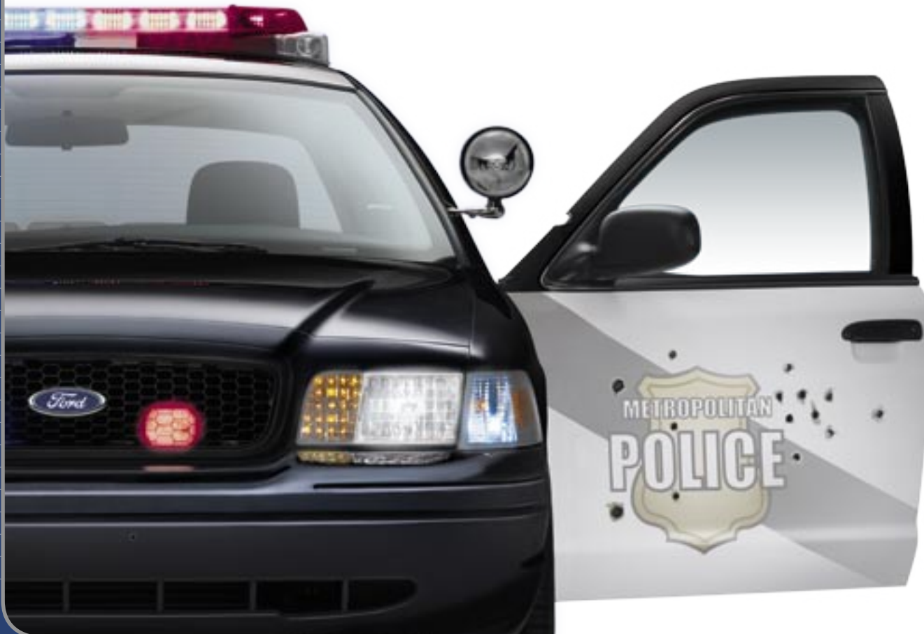
Ballistic Door panel (above) stops the bullets that penetrated the exterior (below).
